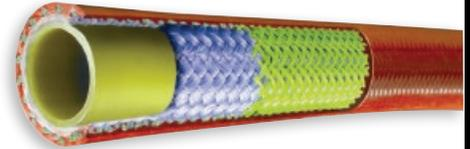
A yellow polyolefin tube, single high tensile synthetic fiber braid reinforcement, rugged polymer belting and abrasion resistant orange polyether-urethane cover.
