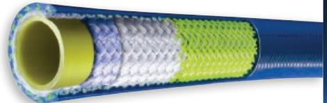
A yellow polyolefin tube, double high tensile fiber braid reinforcement, rugged polymer belting and abrasion resistant blue polyether-urethane cover.
