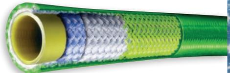
A yellow polyolefin tube, double high tensile synthetic fiber braid reinforcement, rugged polymer belting and abrasion resistant green polyether-urethane cover.
